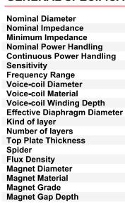
5.5ohm 2000Watts 4000Watts 98dB 35-3KHz 125mm Copper 28mm 400mm In/out 17 Double Silicone 0.98T 280X25mm Ferrite Y30
